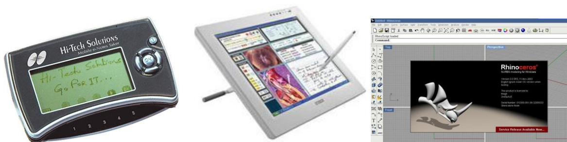
Figure 1. Mobile e-Notes Taker™, Wacom™ DTU-710 Tablet, Computer with Rhinoceros™ CAD
